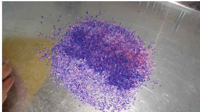
Pour the Silica Gel Desiccant Beads onto a pan such as a cookie sheet. Preheat your oven to 350 degrees. Bake the Silica Gel Desiccant Beads for 45 minutes. Let cool.
