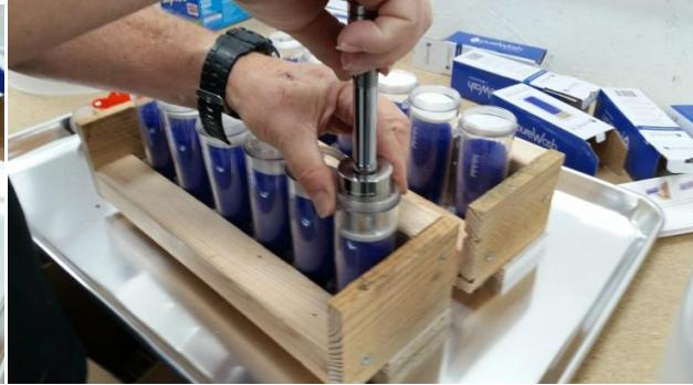
Place one of the larger spacers on top of the Silica Gel Desiccant beads. Using tamping tool, pack the desiccant beads. Note: use whatever you have on hand.
