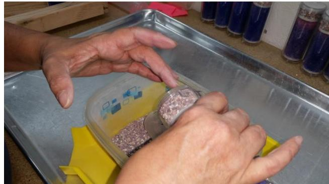
Pour the Montmorillonite Clay Desiccant (gray granules) into a container and set aside.
