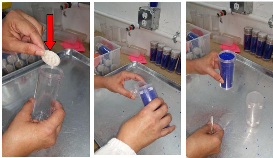
Place the smaller spacer in the bottom of each container. Position the spacer as shown in the picture above (indicated by the red arrow). Using a funnel pour the Silica Gel Desiccant Beads back into the desiccant dryer.
