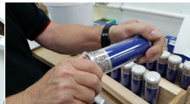
Place the remaining larger spacer on top of the Montmorillonite Clay Desiccant (gray granules). Place the cap onto the container and tighten.
