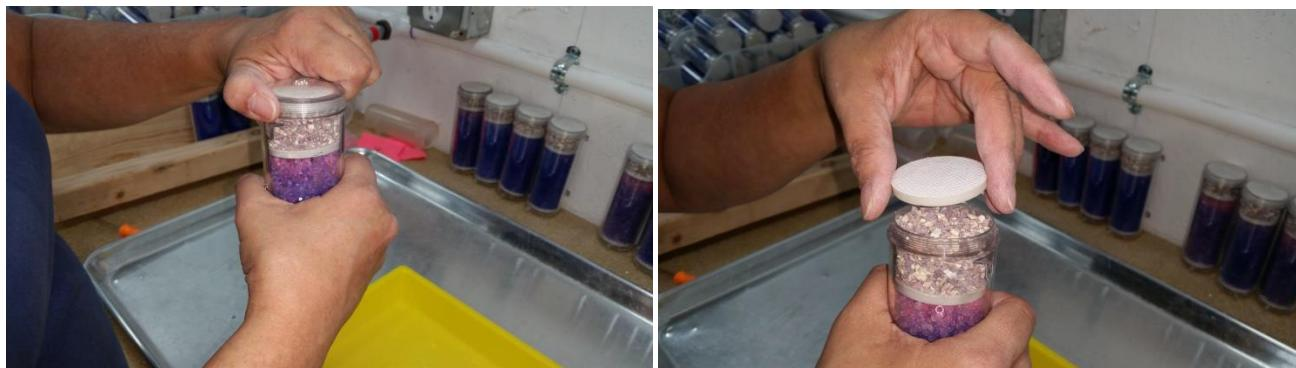
Remove the Desiccant Dryer Cap. Remove the spacer from the top of the Montmorillonite Clay Desiccant (gray granules) and set aside.
