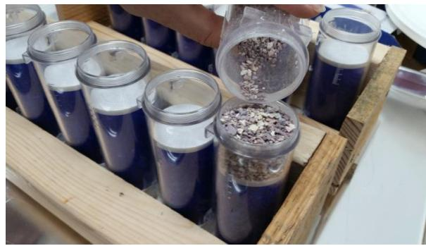
Fill the remaining space in the container with Montmorillonite Clay Desiccant (gray granules).
