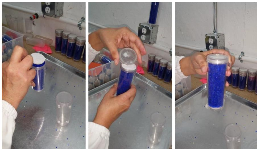
Place the larger spacer on top of Silica Gel Desiccant Beads. Place the cap onto the container and tighten.
