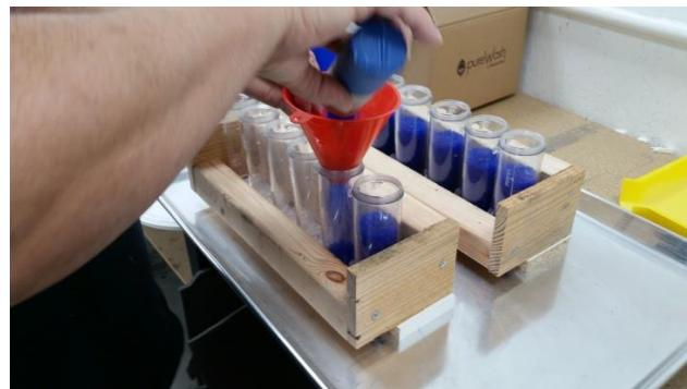
Using a funnel pour the Silica Gel Desiccant Beads back into the desiccant dryer.
