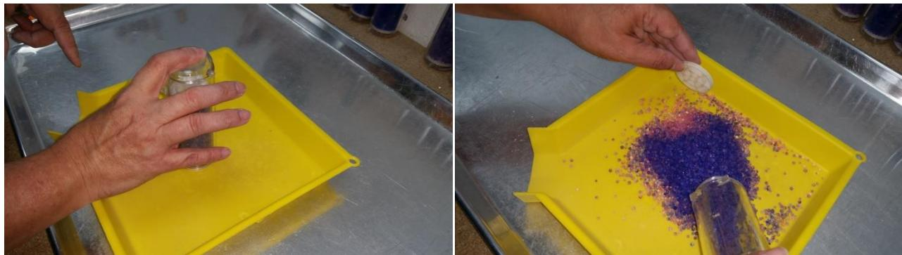
Turn the Desiccant Dryer upside down onto a container (you can use whatever you have) and tap firmly until the Silica Gel Desiccant Beads come out. Remove the spacer and set aside.
