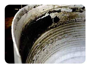
This gunk is **so toxic** that it has the ability to **corrode** through a metal wash wheel, resulting in unnecessary repairs and premature wearing of the washing machine.
